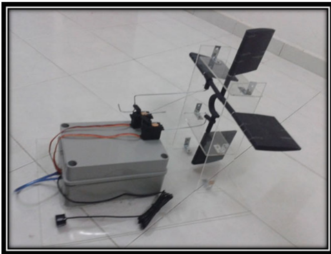
Fig. 5 Components of the hydroplane and rudder
