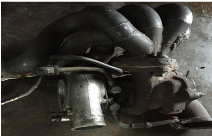
Fig. 13 Turbo and manifold assembly process
