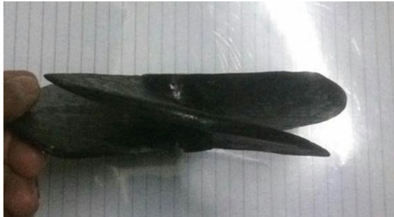
Fig. 10 Complete propeller from 3D printer
