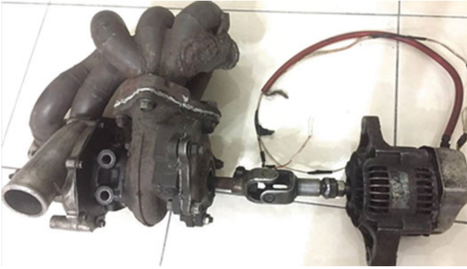
Fig. 15 Complete assembly of electric turbo generator
