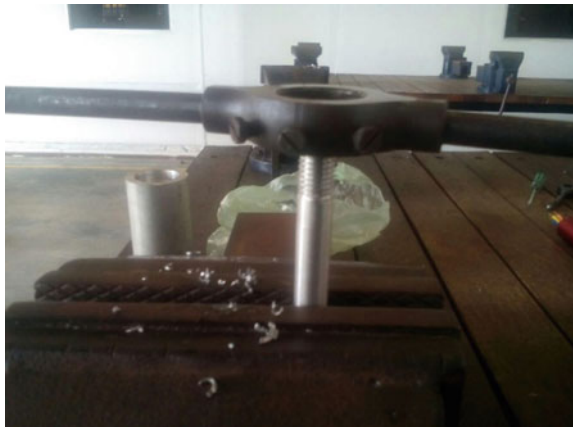
Fig. 11 Process of threading the shaft
