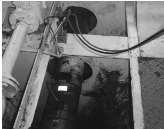
Fig. 13 The set-up of the telemetry system on the output shaft
