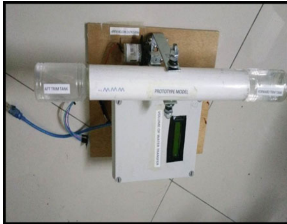
Fig. 7 Prototype design of trim tank control system and the functional test
