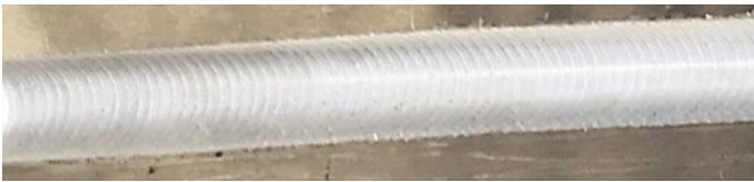
Fig. 6 Welded specimen surface of sample number 4. Smooth welded joint surface; no defects in welded joint (visual inspection); good welded penetration; no flash produced
