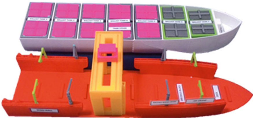
Fig. 12 Prototype of monohull ship floating dry-dock
