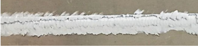
Fig. 4 Welded specimen surface of sample number 2. Poor welded joint surface; severe flash at the side of welded joint; material removal to the side of welded joint; produce wormhole defect along welded joint
