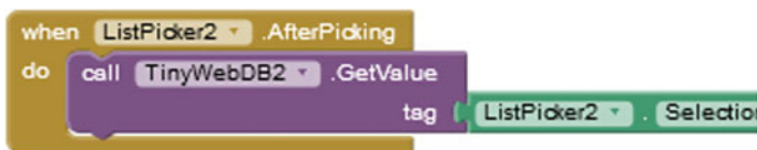
Fig. 2 Blocks component of list Picker and Tiny Web DB
